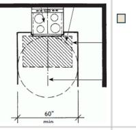
Narrow U-shaped kitchens (lacking a 60-inch diameter turning circle) meet the following requirements:
