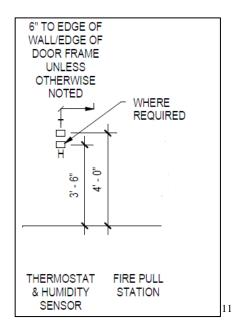
The heights of the thermostats in these inspected units would have been compliant with the 48"maximum height requirement as referenced above if installed according to the plans. But, as built, they are too high, rendering them unusable by persons using wheelchairs.
