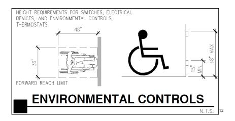
The heights of the thermostats in these inspected units would have been compliant with the 48"-maximum height requirement as referenced above if installed according to the plans. But, as built, they are too high, rendering them unusable by persons using wheelchairs.
