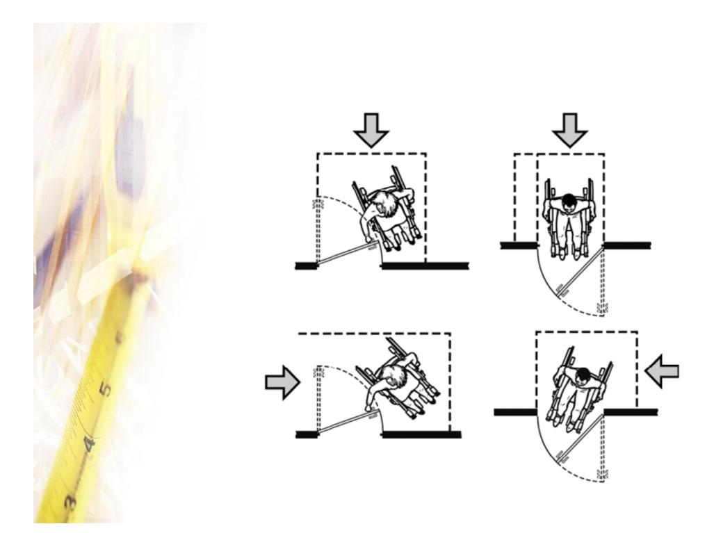
Requirements 3 & 4: Doors sufficiently wide to accommodate wheelchairs and accessible routes into and through each dwelling:
