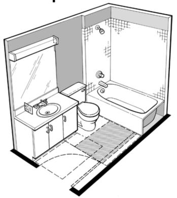
This illustration shows a conventional in-line bathroom design that would comply with Specification "A". A distinguishing feature of a Specification "A" bathroom is that a toilet (or lavatory) is permitted to be located within the clear floor space adjacent to the bathtub. In this illustration a toilet is allowed to be positioned next to the bathtub, making access to the bathtub limited.
