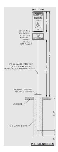
Based on the drawings and instructions above, the height to the bottom edge of the signage designating the accessible parking spaces as reserved for persons with disabilities was designed to be a minimum of 60". However, as built, the heights of these signs result in their decreased visibility that makes it more challenging for persons with disabilities to readily locate these parking spaces.
