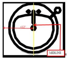
As designed and built, the sink in the bathroom at the Community Room is too close to the wall, rendering this common-use bathroom unusable by persons using wheelchairs.
