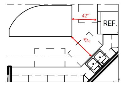
The width of the path around the kitchen island in the Community Room would have been compliant with the 40-inch minimum width if installed according to the plans. But, as built, the path is too narrow, rendering this common-use kitchen unusable by persons using wheelchairs.
